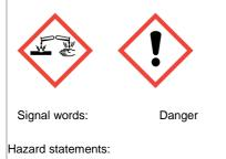
H290May be corrosive to metals.H318Causes serious eye damage.H317May cause an allergic skin reaction.
